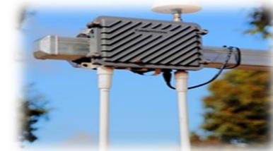
RSU(Road Side Unit)
